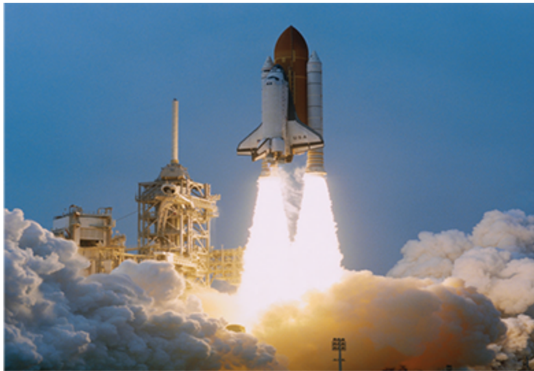
Figure 4.13: Exhaust gases from the booster rockets propel this space shuttle during its launch.
