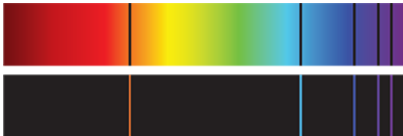
Figure 21.6: The absorption spectrum of hydrogen (top) and the emission spectrum (bottom). The emission lines and the absorption lines are at the same wavelength.
