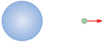
Figure 17.30: The escape speed will take the projectile from a point in the gravitational field to infinity, where it will come to rest.
