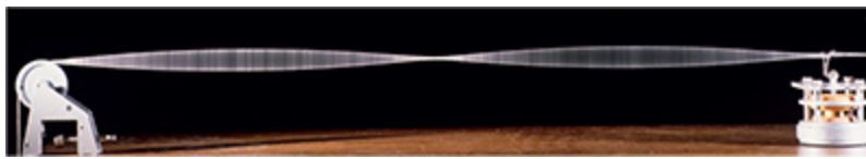
Figure 15.5: This string vibrates in the second harmonic.
