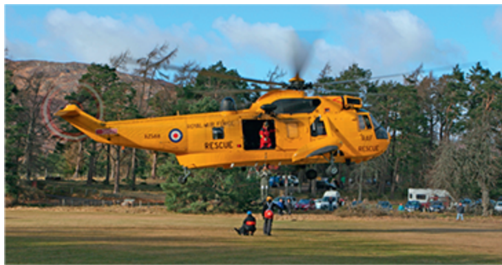
Figure 2.34: The upward force on the rotor is due to the force the rotor exerts on the air downward.
