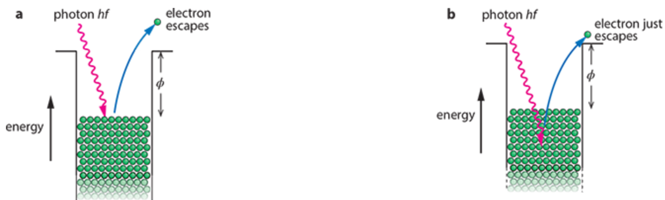
Figure 22.7: a A single photon of light may release a single electron from a metal. b A more tightly bound electron needs more energy to release it from the metal.
